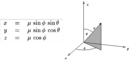
Figure 2-1. Spherical Coordinates
